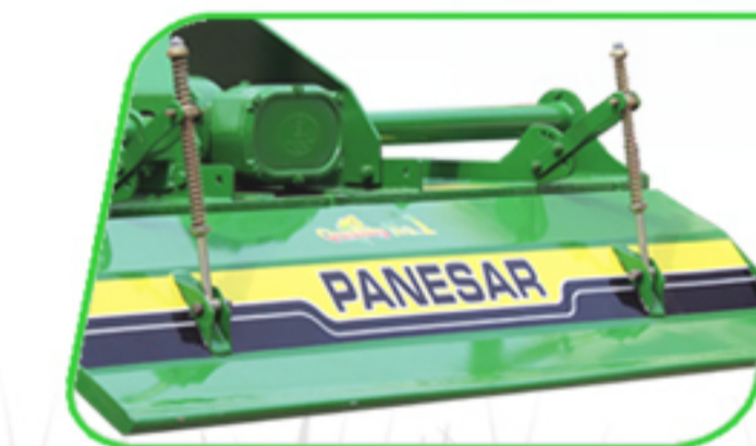
2- RAM springs to adjust the trailing board
